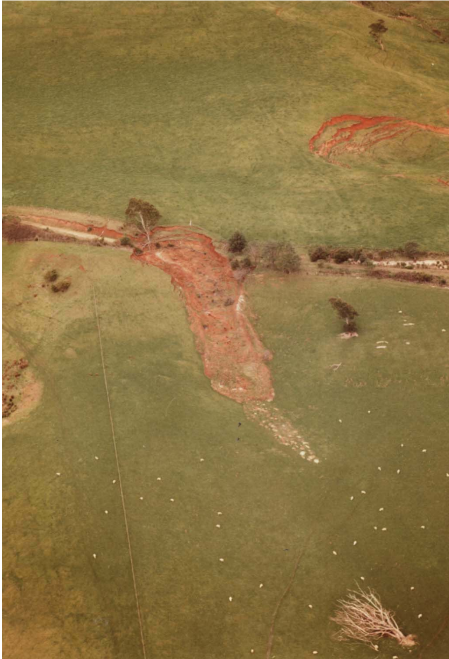
Figure 4.12 – Active slump-earth flow which has removed a section of the Dingley Dell Road. A large tree in the slump zone remains approximately vertical.
