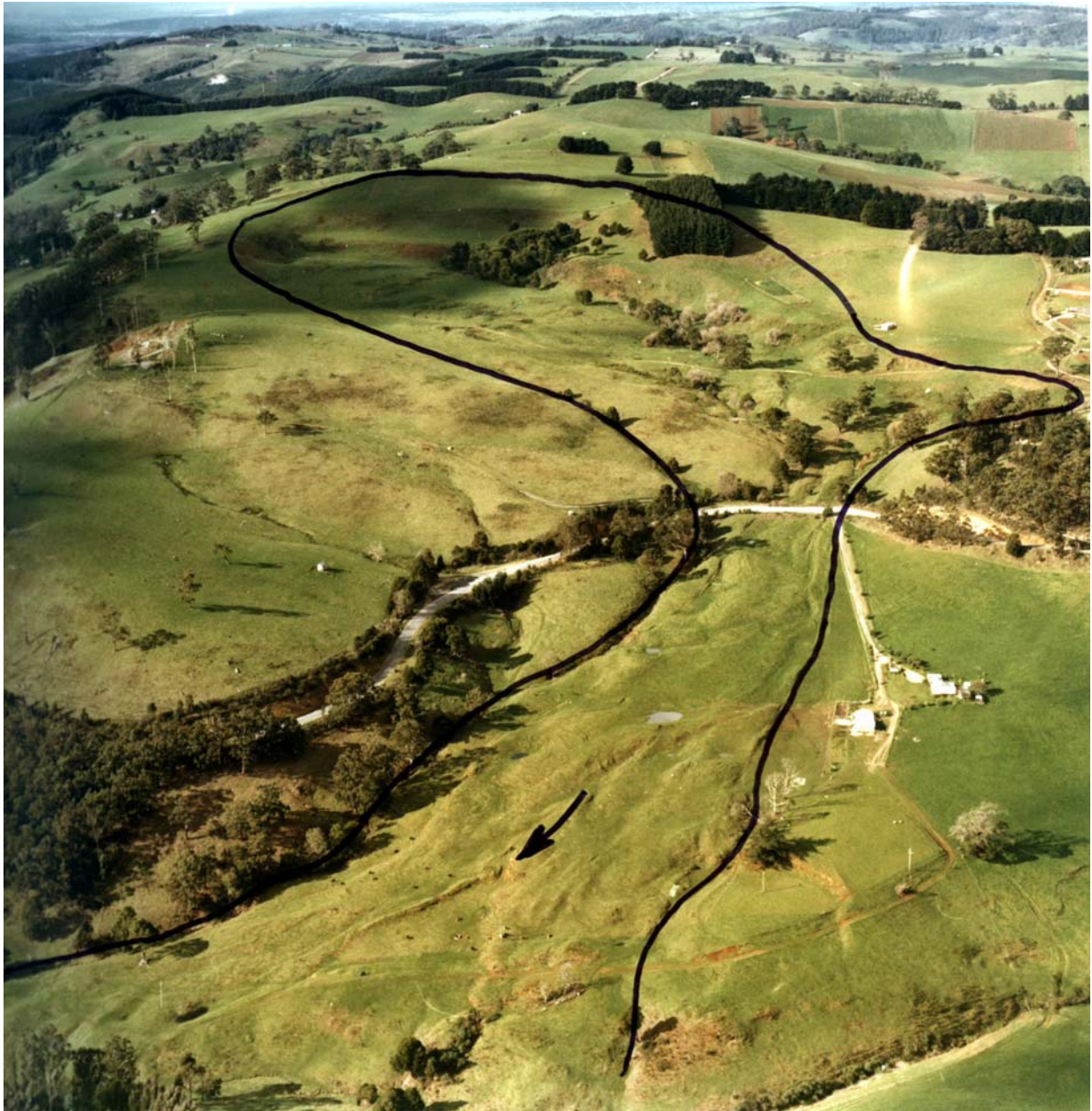
Figure 3.8 – Slump-earth flow cutting across Trafalgar-Thorpdale Road. Slump zone above the road, earth flow zone below road. Winter 1978.
