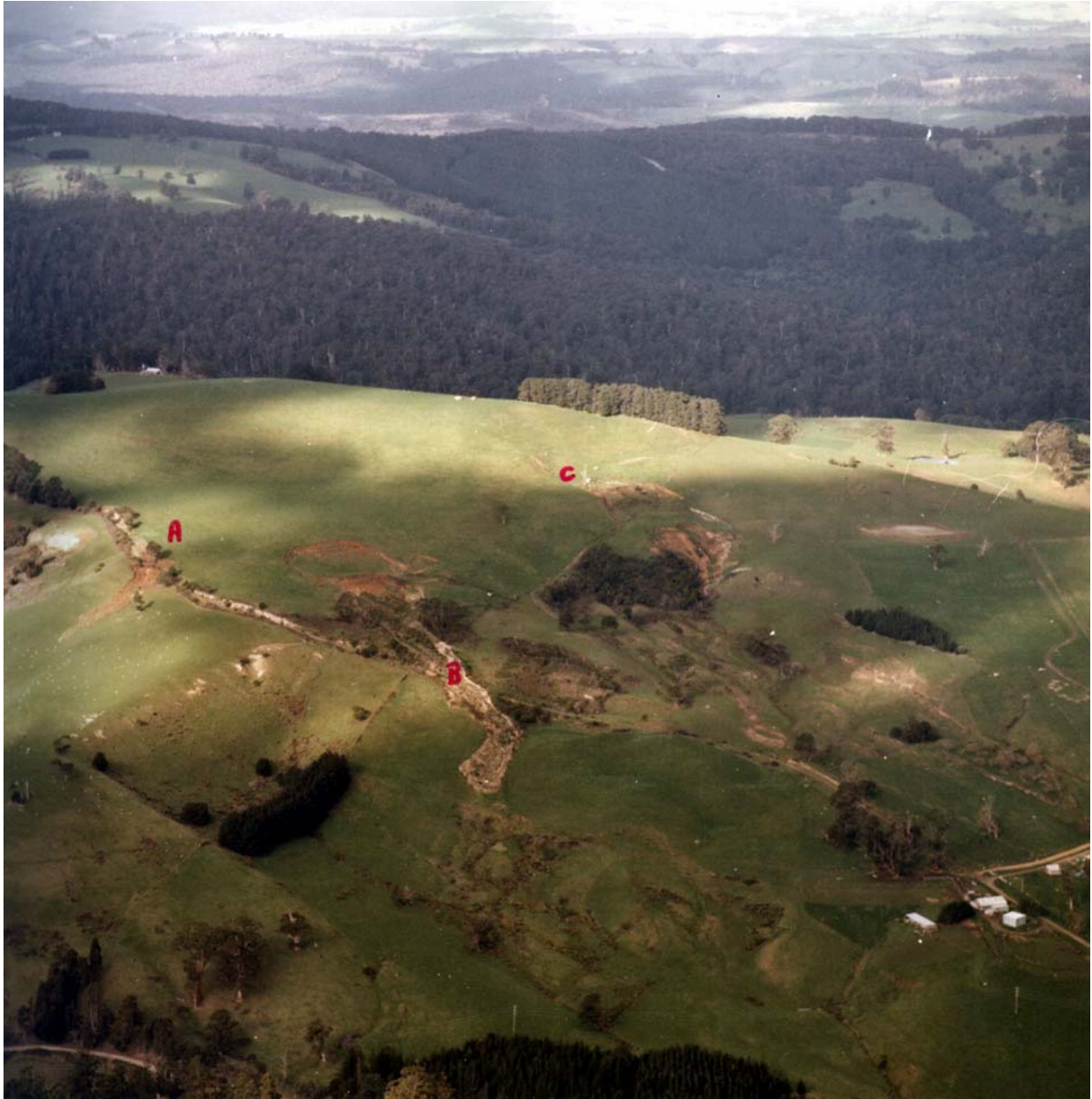
Figure 3.10 – Dingley Dell landslide complex, consisting of at least 3 generations of multiple slump-earth flows.
