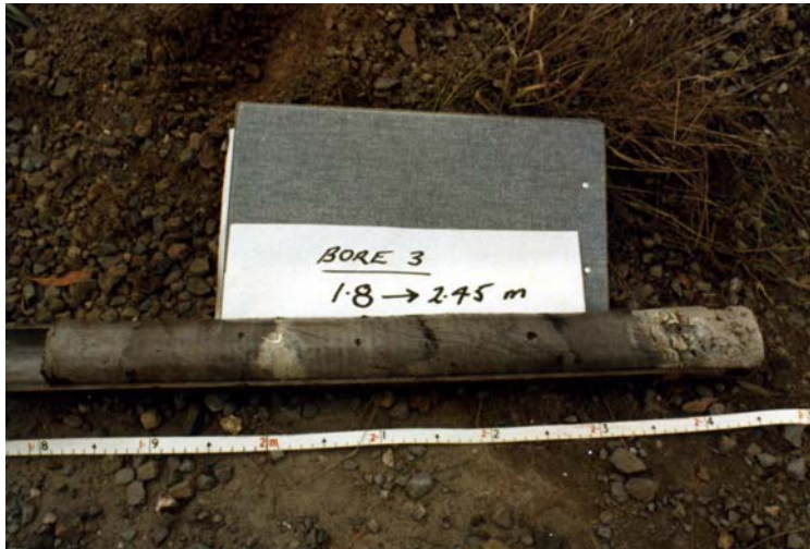
Figure 5.5 - Stiff, pale grey, clay (Ch) (1.80-2.35 m) with carbonaceous seams, plus compact, clayey silty sand (SC) from 2.35 to 2.45 m. Childers Formation, core from bore 3.
