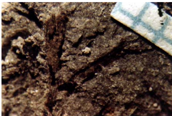
Figure 5.6 – Hard, pale brown, clayey silt, cleaved along original bedding to show fossil plant fragments (Bore 1, Landslide 15, depth 5.0m, magn. 12x). Lower Cretaceous Strzelecki Group.
