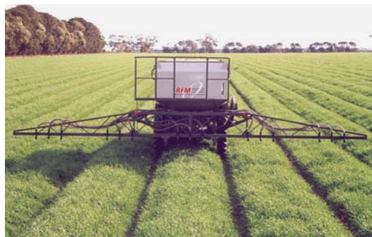
Figure 12. Recent developed machinery ensures the application of fertiliser confined to only the top of beds.
