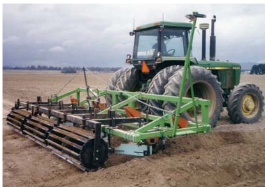
Figure 5. A bed-former used in Southern Australia.
