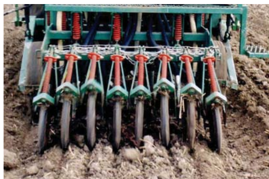
Figure 11. Press wheels ensure improved seed-soil contact and also help in the formation of grooves for water harvesting.
