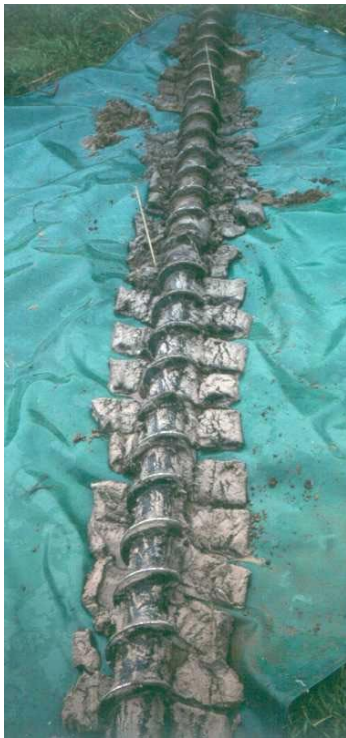
Figure 5. Soil peeled off Gemco auger flights
