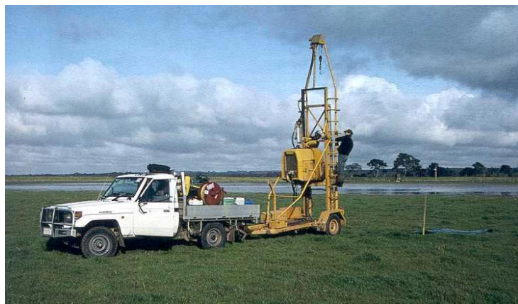
Figure 4. Gemco drilling rig sampling ASS
