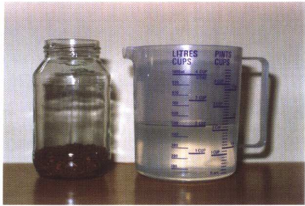
Figure 2. Making up a ratio of 1:5 soil to water (100g soil and 500ml water).
