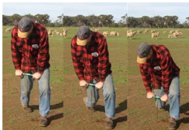
Figure 5. A simple penetrometer indicates soil strength and moisture content.
