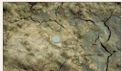
Figure 16 Severe surface crusting occurs when the topsoil is a Type 1 dispersive soil.
