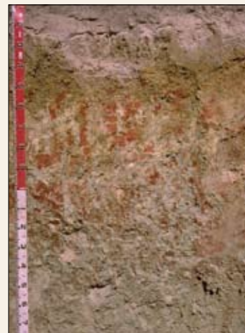
Figure 2 Record the depth where the colour changes down the hole. Note the presence of mottles.
