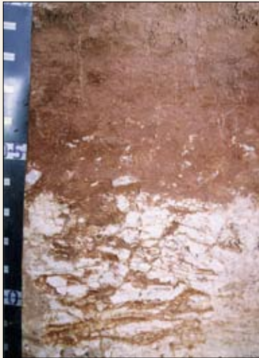
Figure 5 On the Soil Description Recording sheet you will write solid rock at 60 cm. You will write the majority of the roots are at 40 cm. Since there is no obvious colour difference you will record the depths at 10 cm intervals.
