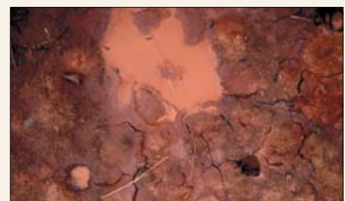
Figure 17 Type 2 dispersion on the topsoil, still leads to surface crusting, but not as severe as a Type 1 dispersive soil.
