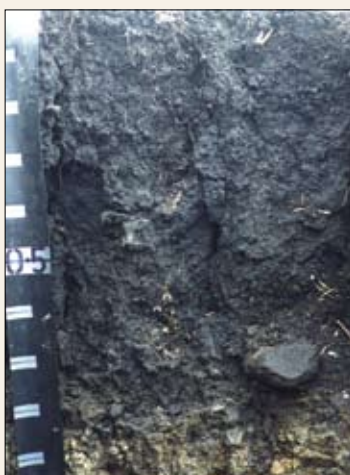
Figure 3 The soil has a similar colour to about 80 cm but the structure of the soil changes at 20 cm and again at 60 cm, therefore you would identify these depths as the different layers.
