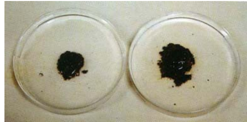
Figure 21 – Aggregates showing slaking. Form left: minimal and significant
