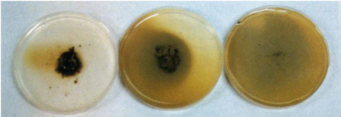
Figure 22 – Petri dishes showing dispersion levels. From left: little or none; incomplete and complete dispersion
