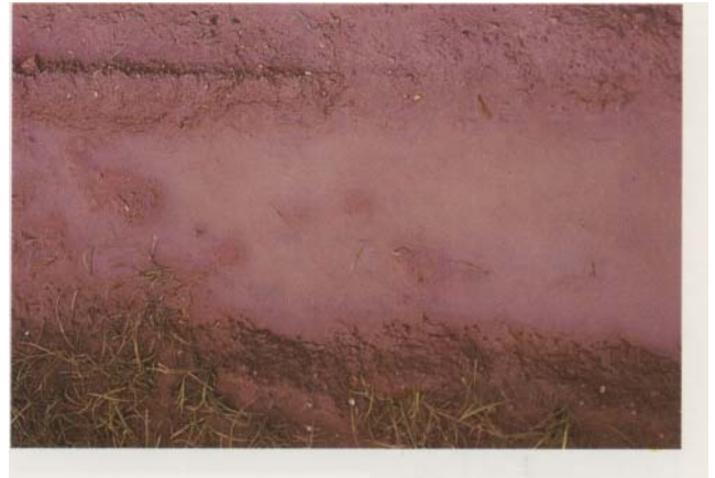
Figure 21: Dispersed clay in a puddle.
