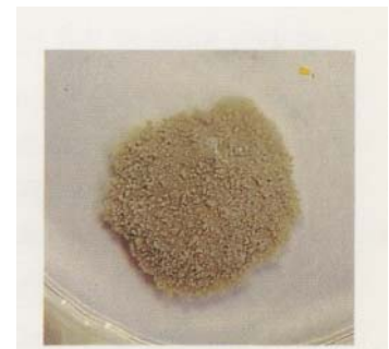
Figure 24: An aggregate that has slaked into smaller aggregates or microaggregates.
