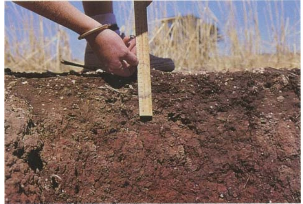
Figure 9: Measuring topsoil depth.
