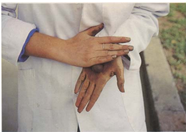
Figure 17: Kneading the soil to form a soil texture ball.
