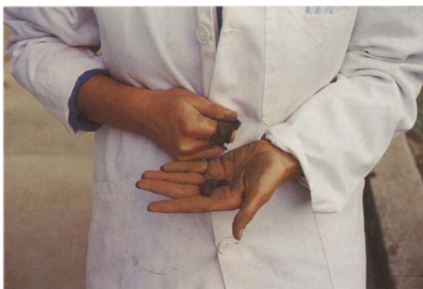
Figure 18: Ribboning the soil ball between thumb and forefinger.
