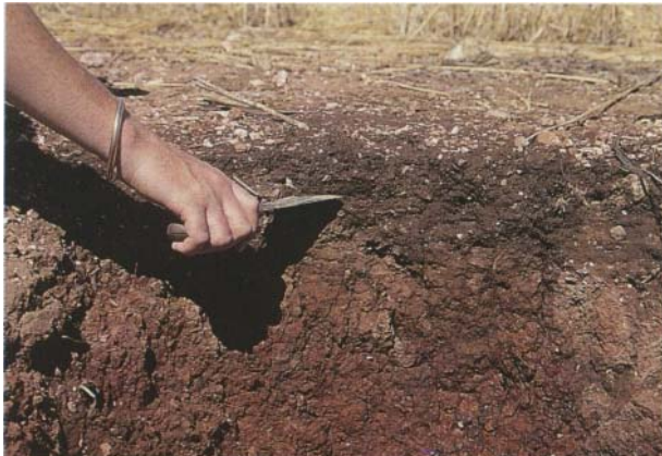
Figure 5: Use the spatula to flick out soil to expose an unsmeared soil profile.
