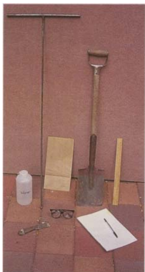
Figure 3: This is all the gear you will need to assess the structure of your soil.
