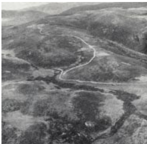
Plate 36. The High Plains land system between Mt. Nels and Spion Kopje. The race-line which runs across the centre of the picture diverts water from the High Plain's section of the Big River (Mitta Mitta) across the catchment boundary into the East Kiewa River
