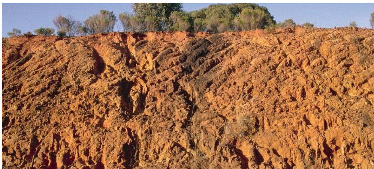
Plate 9 The Parilla sand is close to the surface on the crest of the Diapur Ridge. Parilla sand is partially ferruginised forming a weak sandstone that is used as substrate for roading in the region.
