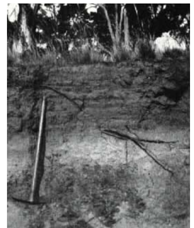
Plate 24 – One indication of serious erosion is deposits of silt overlying the original ground surface. Here, about two feet of silt is exposed in the wall of a gully. The A horizon of the original soil is the white band across the centre of the picture
