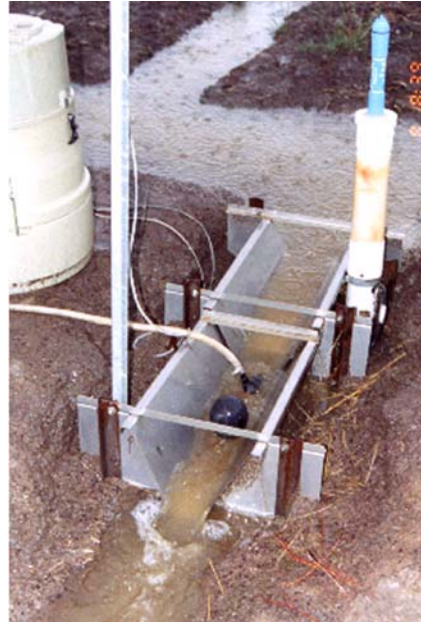
Water being automatically sampled in a flume in February 2002.
