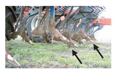
Elevate the tines and block hoses behind wheels to leave wheel tracks bare. Spray tracks in particular are best to be left bare to provide better in-crop guidance.
