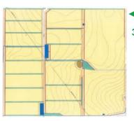
With a contour survey, a whole farm plan is simplified. Paddocks suitable for beds can now be identified, water movement planned, vegetated waterways and buffer dams located. The really wet ar-
