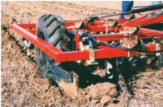
To accommodate bed renovation (and perhaps bed making) furrowers have been fitted to the front tool bar.
