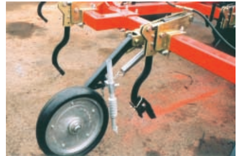
Knife points, press wheel depth control and spring sowing tubes have been incorporated. Also hydraulic rams are used for the opening tines and points.
