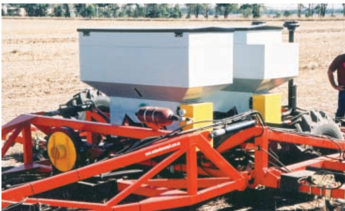
Two air boxes with 880 litre capacity fitted over the tool bars. Small air boxes are fitted to reduce the temptation to carry too much weight in wet conditions.
