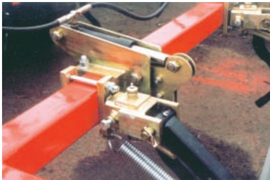
Note the opening tines and press wheel assemblies are attached to the tool bar separately.
