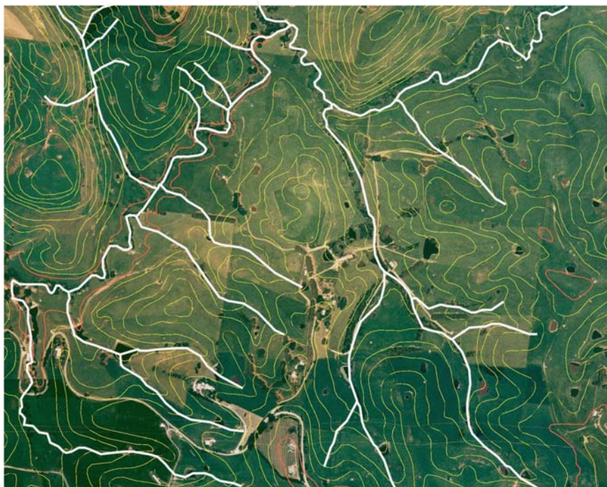
Fig 3 Orthorectified vertical aerial photograph taken November 2002, showing 10 metre contours and drainage lines.
