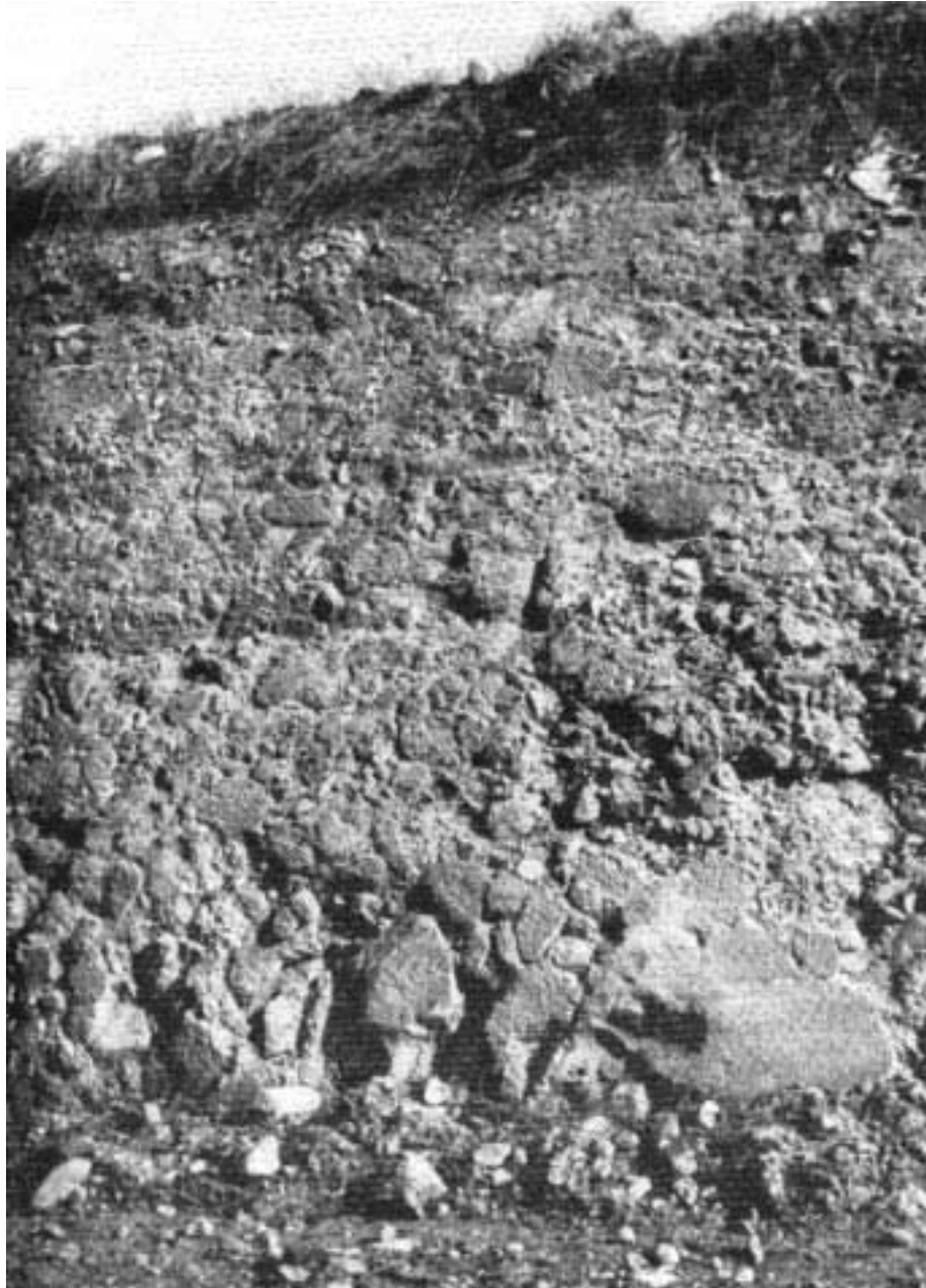
Plate 3 - Highly weathered colluvium exposed in a road cutting at Gundowring South. The largest fragments are more than a foot across
