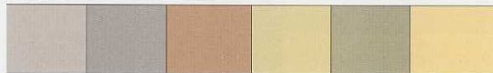
Diagram 1 Pale soils. If any of these colours approximate the topsoil colour, then the topsoil is considered pale.
