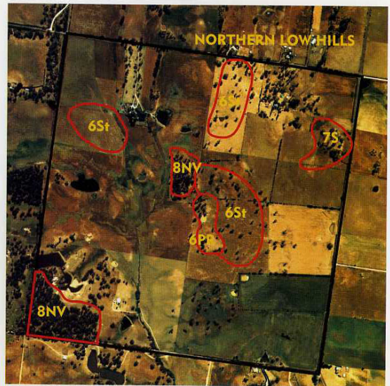
Figure 10 Step 5: Marking out and labelling areas of high rock outcrop or surface stone on the plan.
