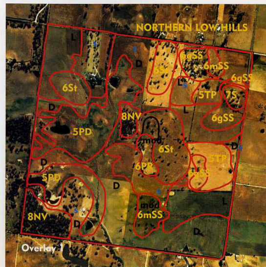
Figure 26 Step 10: Marking out the boundary between shallow topsoil and deep topsoil in each of the landscape areas on the plan. When in place, the overlay shows the landscape code (in black) and the depth of topsoil (in blue).
