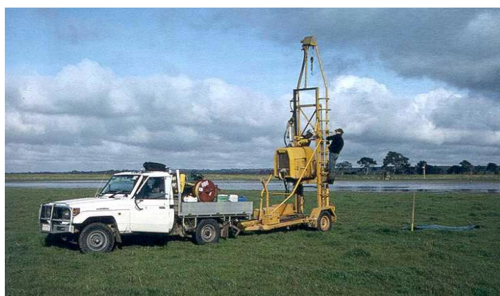
Figure 4. Gemco drilling rig sampling ASS
