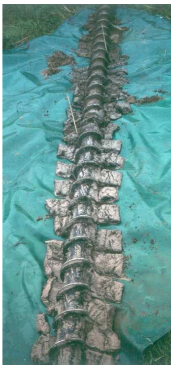
Figure 5. Soil peeled off Gemco auger flights
