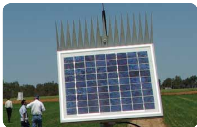
Solar panel unit for SMM data logger
