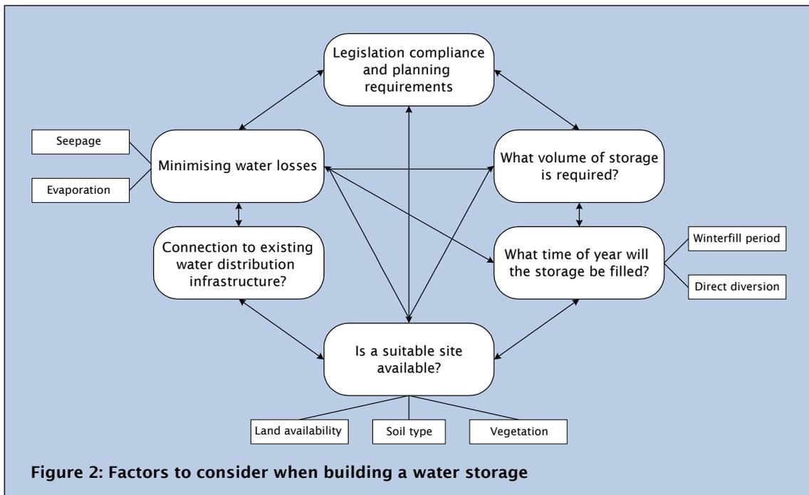
**Figure 2: Factors to consider when building a water storage**
