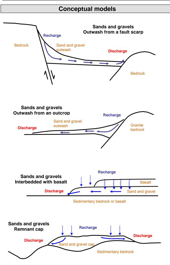
A variety of conceptual models for salinity processes in different geological settings. The common theme is the lateral flow of groundwater through the sand and gravel GFS.
