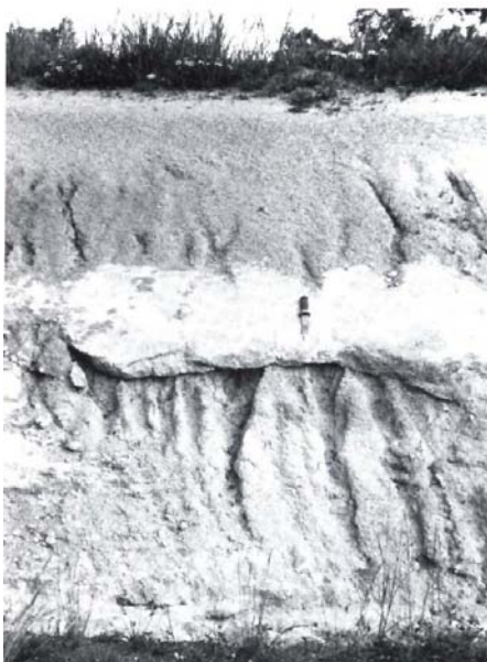
Hardpans at approximately one metre depth restrict water movement and root penetration to the lower soil profile.
