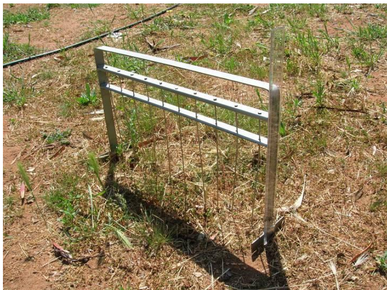
Figure 2: Levy point sampler used for assessing vegetation cover.
