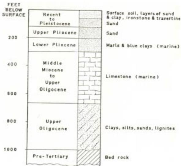
**Fig 3 – Generalized section of a Mallee Bore.**
