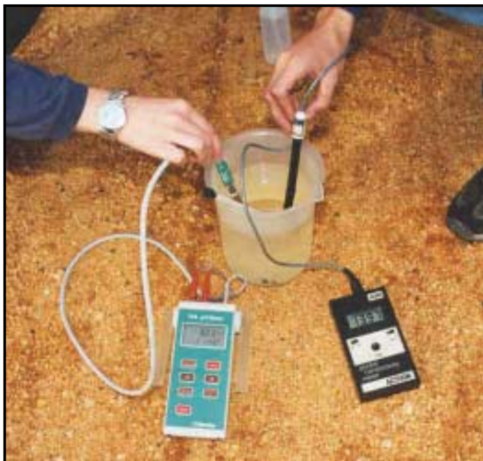
*Figure 2 showing field testing for pH and EC.
