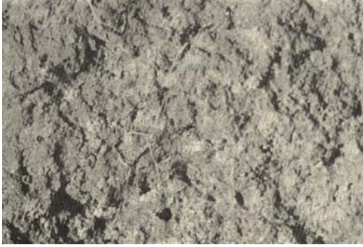
Plate 2 – K2 silty clay (subsoil) showing matt face and visible pores (x6).
