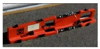
Figure 6.6: Geonics EM38 conductivity meter (www.ussl.ars.usda.gov).
