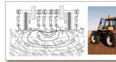
Figure 6.5: A cross-sectional representation of the VERIS 3100 in operation (www.veristech.com). Electrical arrays are created by pulsing a current through the coulters to record the average concentration of salts to 30 and 90 cm.
