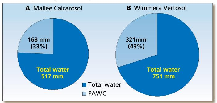
Figure 2.4: Comparison of total soil water storage and plant available water capacity (PAWC) for (A) Mallee Calcarosol and (B) Wimmera Vertosol, assuming a rooting depth of 150 cm.
