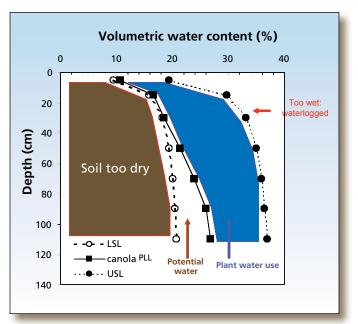
Figure 2.2: Diagrammatic representation of water use by canola growing on a Calcarosol from Birchip, Victoria. The diagram shows the total actual amount of water that can be used by the plant (PAWC) referred to as 'plant water use' on the graph. The soil water listed as 'potential water' is the quantity of water unavailable to crops due to subsoil constraints. The sum of 'plant water use' plus 'potential water' equates to the PAWC<sub>E</sub>.
