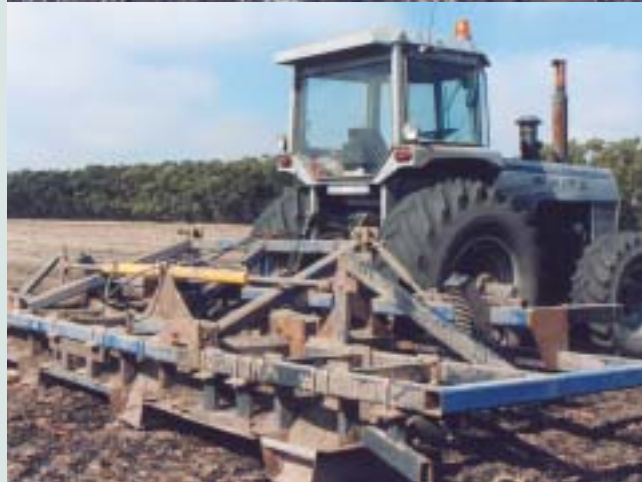
Machines used in raised-bed renovation.
