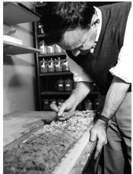
Figure 5. After transporting of the harvested monolith back to the laboratory, "picking down" carried out following some strategic drying.
