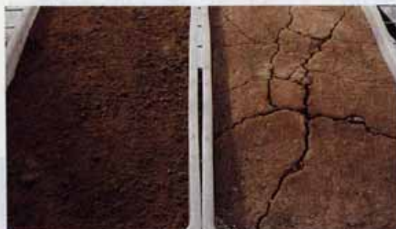
Persistence of original structure when treated with gypsum
