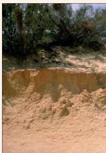
Figure 7 Sandy soil, located in a low rainfall area. The Drainage column of the Summary Recording Sheet would be shaded red for this soil type (due to excessive drainage).
