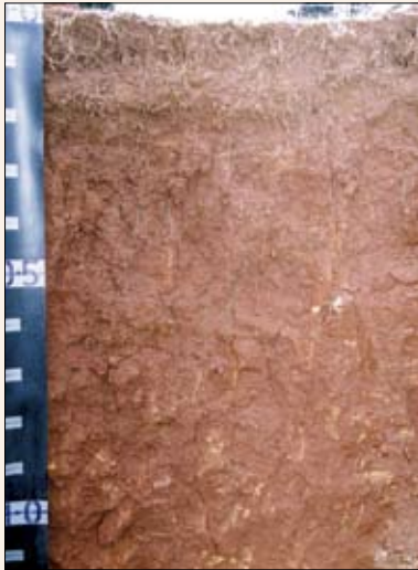
Figure 9 Red subsoil, no mottles or pale layer, Structure column is shaded green. The drainage column of the Summary Recording Sheet would be shaded green for this soil type.
