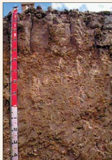
Figure 3 The majority of roots are in the topsoil (0-10 cm). The friability is hardsetting from 10-50 cm. This layer is highly dispersive (Type 1). The Structure column of the Summary Recording Sheet would be shaded red for this soil type.
