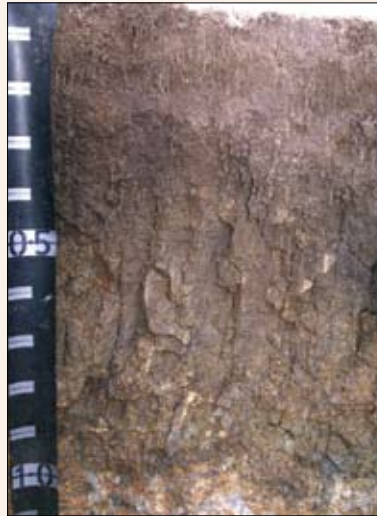
Figure 10 Brown subsoil, no mottles or pale layer, Structure column is shaded green. The drainage column of the Summary Recording Sheet would be shaded green for this soil type.
