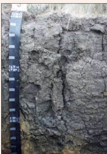
Figure 6 Grey soil, Structure column is shaded red, subsoil very clayey. The Drainage column of the Summary Recording Sheet would be shaded red for this soil type (due to poor drainage).
