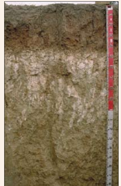
Figure 1 The topsoil is darker in colour and light textured while the subsoil is brighter in colour and heavy textured.
