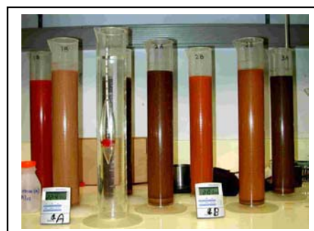
Photo 5.4 Hydrometer Measurement for Texture Analysis
