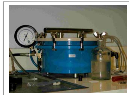
Photo 5.3 Pressure Plate Extractor Apparatus
