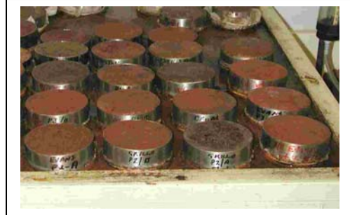
Photo 5.1 Saturation of Soil Core by Capillary Flow
