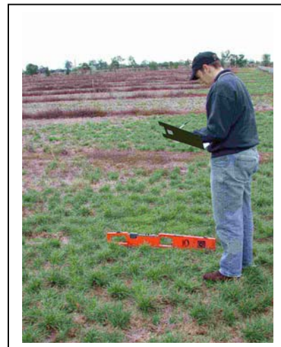
Photo 4.5 EM Measurement using EM38 Instrument
