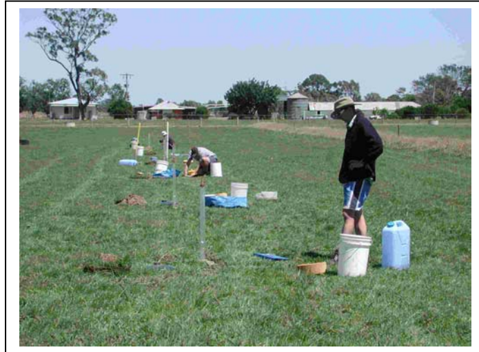
Photo 4.6 Field Measurement of Hydraulic Conductivity in Grid Row
